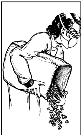
Figure 2: Wear protective clothing when installing insulation.
