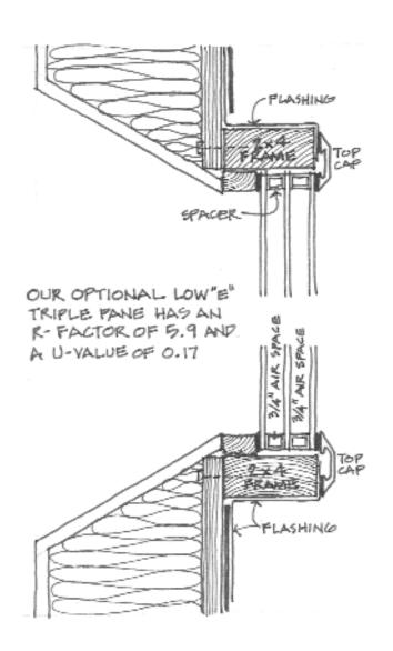
Natural Spaces insulated glass windows are available in double, triple and four pane systems. We use 3/16"" and thick tempered glass, which is 5 times stronger than plate glass. Our skylights have made it thru hail storms where conventional 1/8" thick tempered glass skylights were blasted out. By using glass instead of plastic, our
